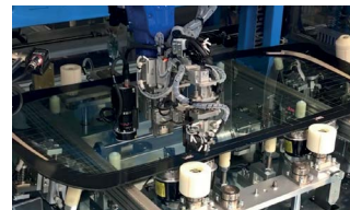
Automatic terminal soldering system for automotive glass
